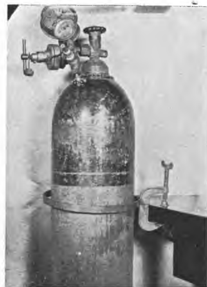
Figure 6. One method of securing a compressed gas cylinder against falling. (See paragraph 49.)
