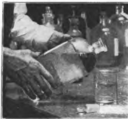
Figure 7. If the stopper of the bottle is laid on the bench as shown at the left, it may become contaminated, thereby causing fires, burns to the chemist, or other mishaps. These will be avoided if the stopper is handled as shown at the right. (See paragraph 61.)
