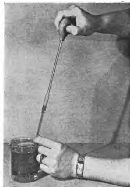
Courtesy Hercules Powder Co. Figure 10. A suction bulb used for filling a pipette. (See paragraph 68.)
