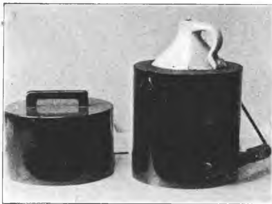
Courtesy Westinghouse Electric & Mfg. Co. Figure 13. Well-designed container for small quantities of acid. This consists of a gallon jug which is set in a metal pail and then surrounded with asphalt compound. A stopper should be provided for the jug and a cover for the metal pail. (See paragraph 69.)
