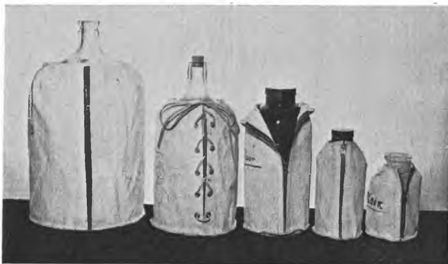
Figure 14. Canvas jackets for carrying acid bottles. (See paragraph 69.)
