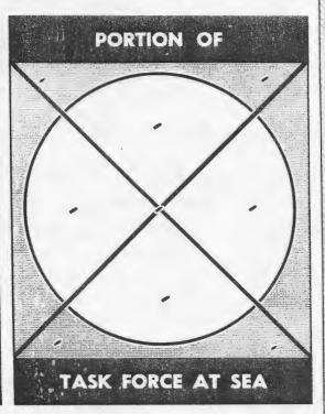
ARRANGEMENT AND CONCENTRATION OF SHIPS AT BIKINI INSURES GRADUATED DAMAGE
